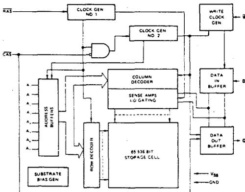
NOTE: The following IEEE STD. 662-1980 symbols are used in this data sheet: D = Data In,  $\bar{W}$  = Write Enable, Q = Data Out.
