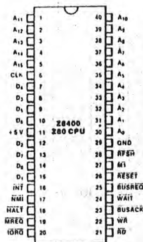
Figure 2a. 40-Pin Dual-In-Line Package (DIP) Pin Assignments
